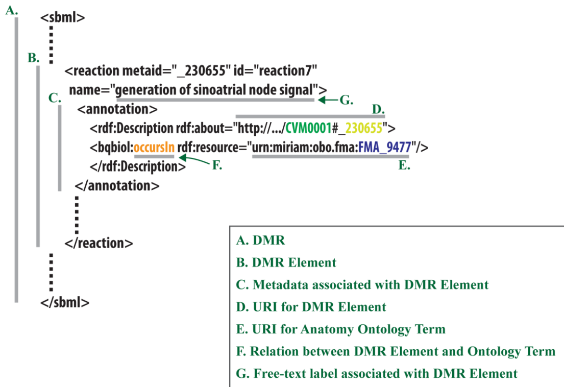
Figure 2. Example illustrating the structure of an archetypal model resource A (in this case, an SBML model) in which element B is shown to bear (i) a human-readable text label G , as well as (ii) machine-readable metadata C . The annotation in the metadata above conveys the meaning that the reaction with the Unique Resource Identifier ( URI ) 230655 ( D ) that occurs in ( F ) the anatomical location identified by URI E . The latter URI represents the sinoatrial node term in the Foundational Model of Anatomy.
